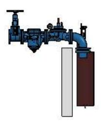
If the inlet pressure is between 4 to 9 bar, an orifice is required after the Hawido valve. The pressure will be reduced in two steps.
