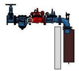
If the pressure is between 9 to 16 bar, a Hawido pressure reducing valve is required before the floating valve.
