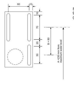
Slot width: 9mm for M8 screws (use only corrosion-resistant screws)
