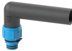
Elbow 90° with ZAK® spigot end and PE fusion end for water d32, d40 ZAK34 / d32 - d63 ZAK46 / Gas d32, d40 ZAK34 / d32 - d50 ZAK46
