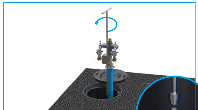
Use the operating key to bring the hydrant in opened position by approx. 15 revolutions (hand-tight).
